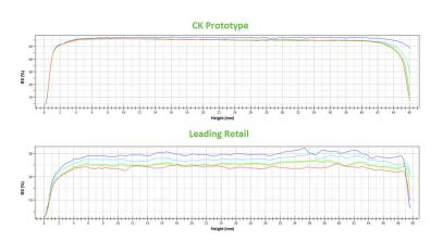
The above graph compares the backscattering results measuring the uniformity of droplets and suspesion of solids of a CK prototype waterless hand cleaner with grit vs a leading waterless hand cleaner with grit. Uniformity is key in ensuring consistency in product and usage.
